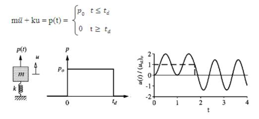
With at-rest initial conditions: u(0) = u(0) = 0. The analysis is organized in two phases.
