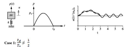
Forced vibration phase: The force is the same as the harmonic force  $p(t) = p_0 \sin \omega t$  considered earlier with frequency  $\omega = \frac{t_d}{T_n}$ .
