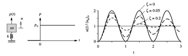
Where  $(u_{st})_0 = \frac{p_0}{k}$ , the static deformation due to force  $p_0$
